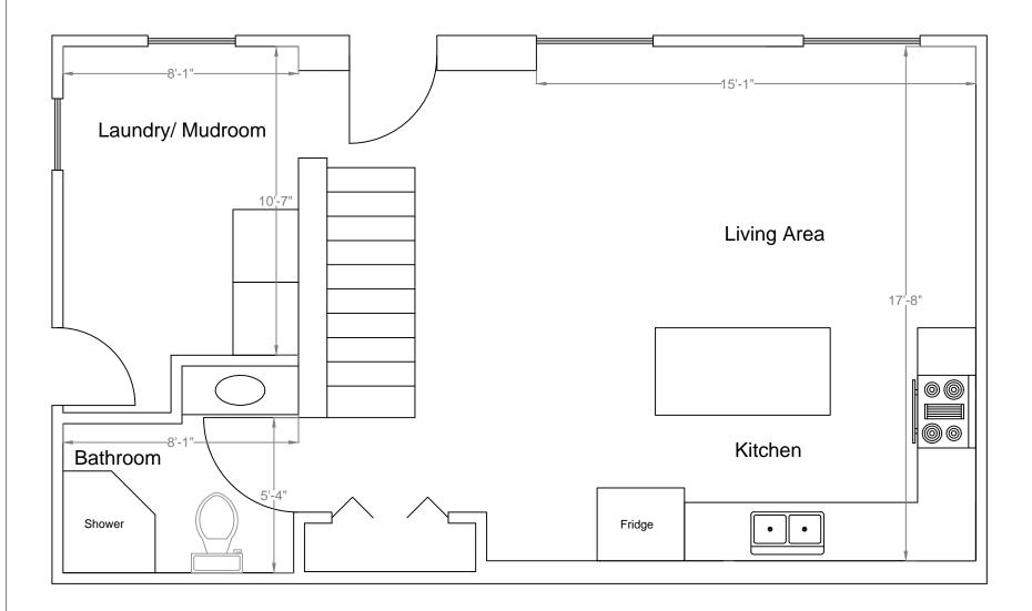
Exterior walls to be insulated with R-14 Roxul Smoke Detector/Carbon Monoxide Detector to be hardwired and connected to detectors on each subsequent floor Electrical work to be ESA compliant with seperate permit
